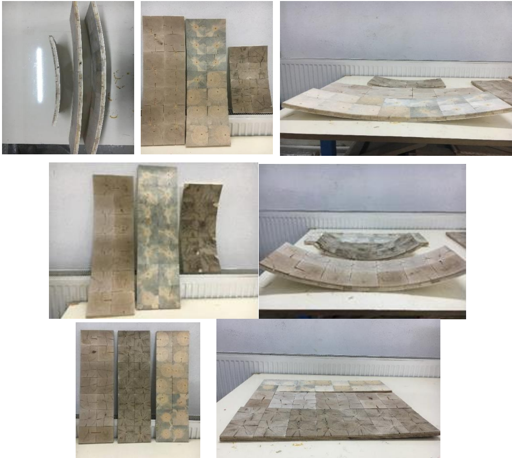
Figure 5. Type 1 End grain laminated parquet production result
