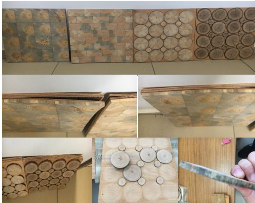
Figure 6. Type 2 End grain laminated parquet production result
