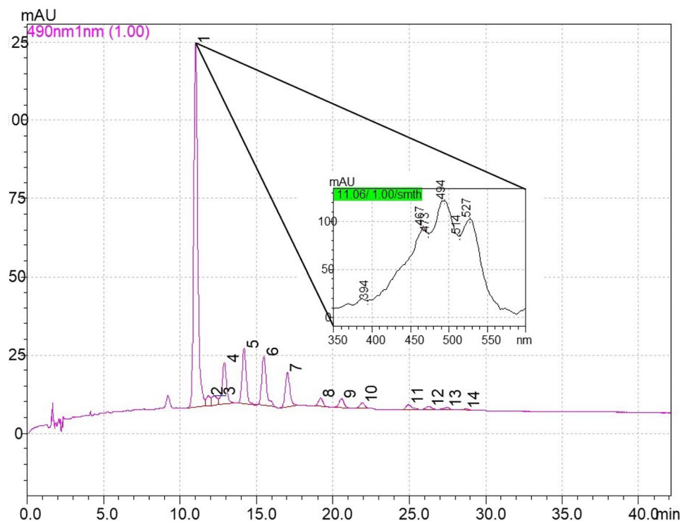
Fig. 5 HPLC (Shimadzu LC-20A Prominence) chromatogram of carotenoid extract from Haloterrigena thermotolerans K15 and spectrum scanning of the all-trans bacterioruberin
