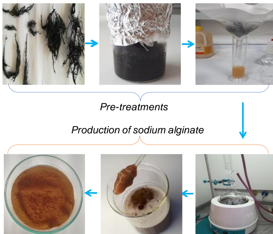
Figure 5. Sodium alginate production process from brown algae.
