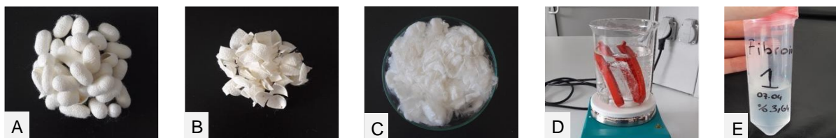
Figure 1. Production steps of silk fibroin. A. Bombyx mori cocoons B. Dissections C. Fibroin fibers after removing the sericin D. Dialysis in the bi-distilled water after solving in LiBr solution E. Pure fibroin solution.
