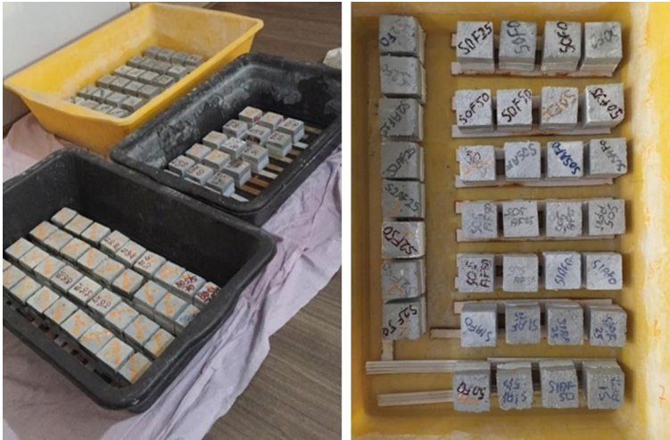
Fig. 5 Sorptivity test of mortars
