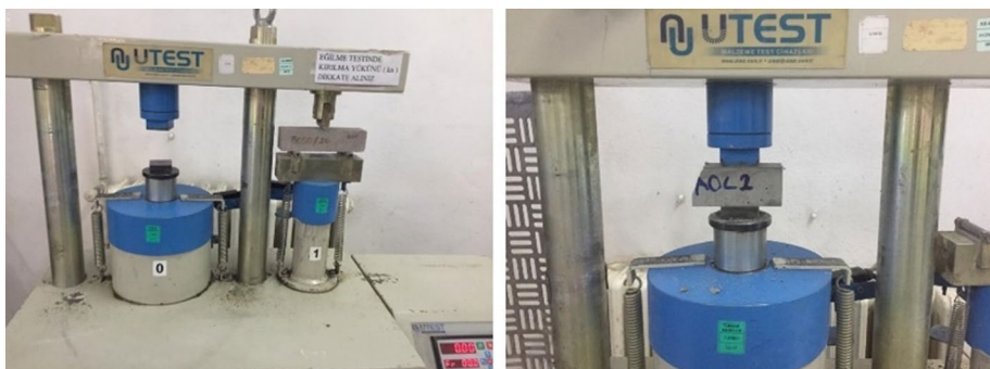
Fig. 3 Compressive and flexural strength tests which are applied to mortars
