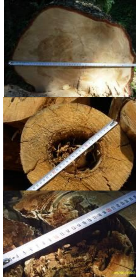
Fig. 1. Types of heart rot (healthy wood, spongy wood, rotten wood)
