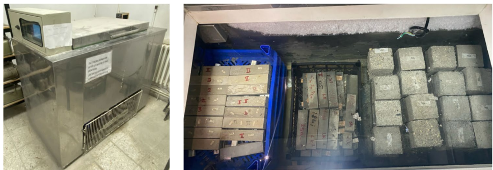
Fig. 7 Freeze–thaw test setup
