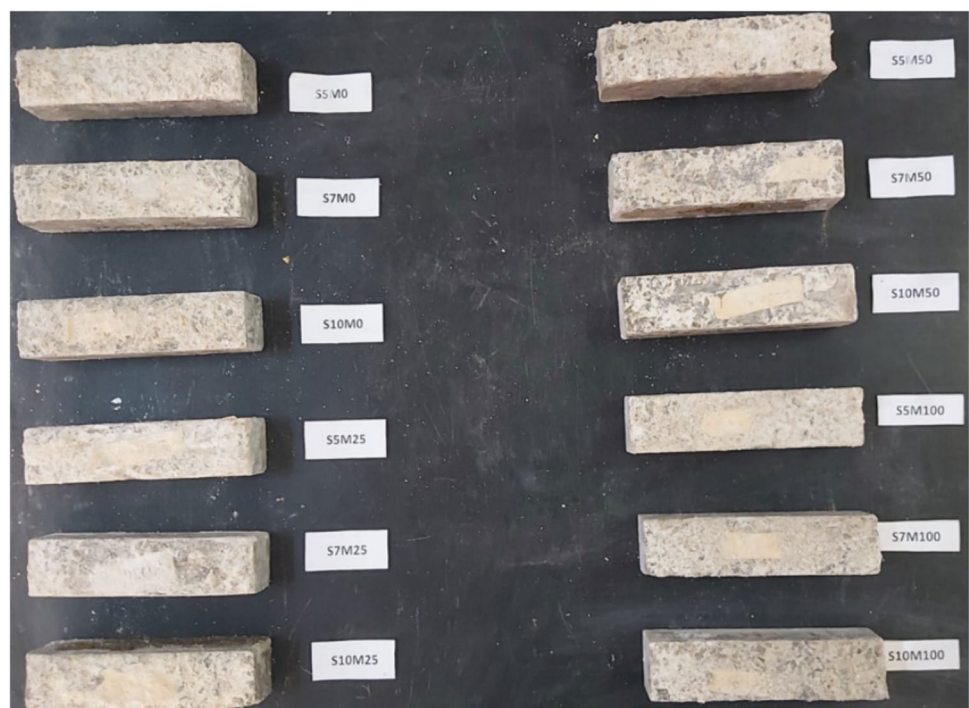
Fig. 14. The images of samples after the \text{Na}_2\text{SO}_4 effect
