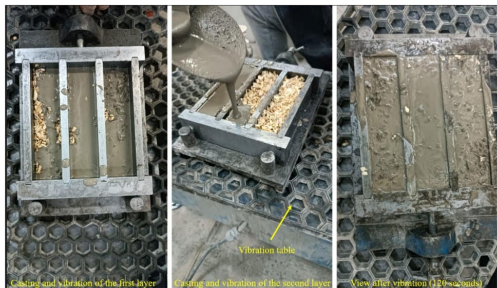
Fig. 3 Production stages of prepacked composites
