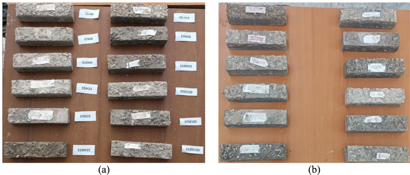
Fig. 19. The images of samples after a 30 cyclic and b 60 cyclic freeze–thaw tests
