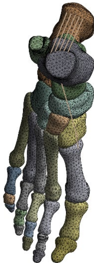
Figure 3. Finite element mesh structure of the foot model.
