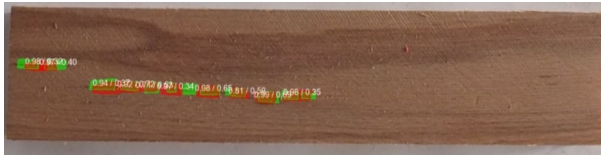
Fig. 11 Prediction and masking of the crack model after 150 iterations
